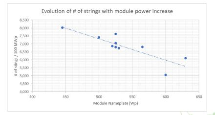
Note: String lengths calculated based on a Min Site Temp of -20C
